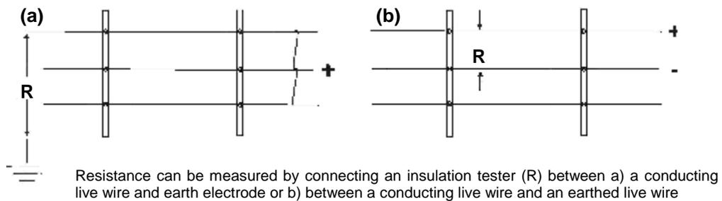
When the fence erection is complete, the total insulation resistance of the fence should be measured with the energiser disconnected (Figure 12). A reading on the insulation tester in excess of 2 megohms indicates an acceptable level of insulation between the conducting wires and earth.
