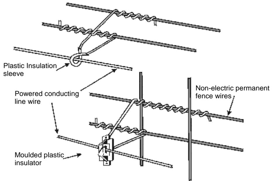
Plate 2 - Metal fence stake with adjustable insulators
