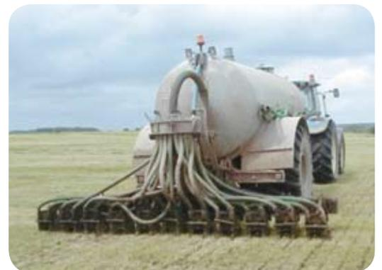
Figure 2. Slurry application using trailing hose and shallow injection equipment
